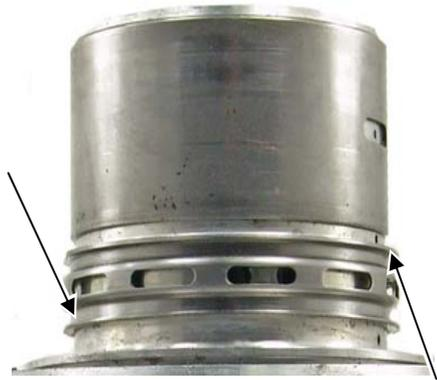
The arrows are pointing to the outside of the ring grooves where the rings need to seal. This is the area where the bronze particles accumulate and imbed into the support.
