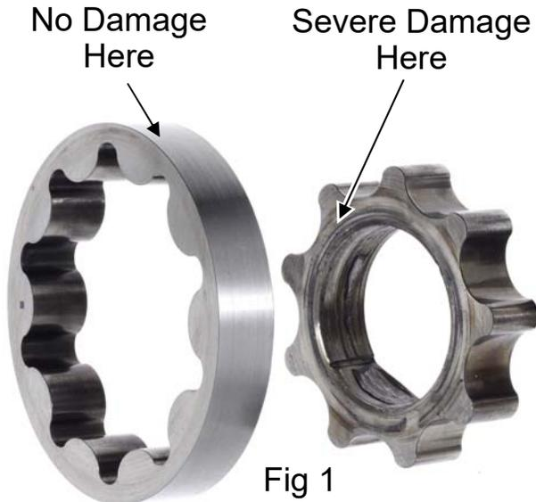
Electrical ground failure or a tight pump bushing clearance will weld the inner gear to the pump plate.
