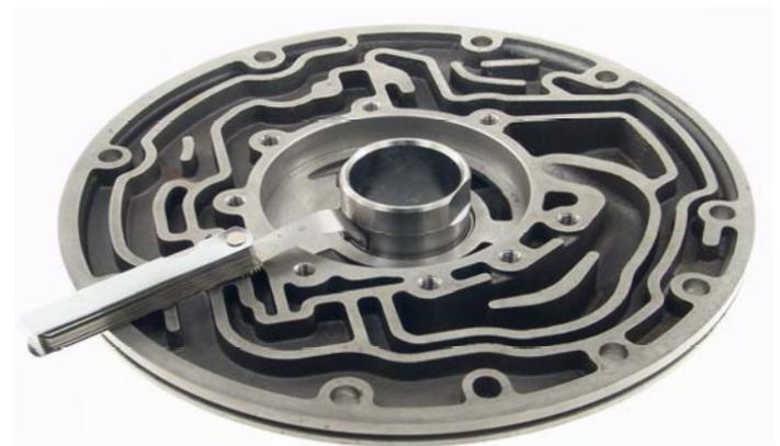
We have heard the reports of replacement bushings that will only provide .001" clearance to a properly sized hub. Running the bushing this tight will seize the bushing to the hub and spin the bushing in the pump body. The metal generated will get between the inner gear and pump plate welding them together, this will look like a ground failure, see fig 1. Tolerances and alignment are critical with this pump. See TransGo 5R1-PMP-Align.
