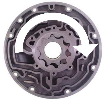
**Line Pressure and Pump Failure:** Aggressive computer programming can contribute to high line pressure and pump failure, see page 1 fig 2. Check with a pressure gauge during the road test. Stock Programming: Light-load cruising speed 150-170psi and very reactive to engine load. Hard throttle up-shifts 200-235psi. Full throttle starts can briefly spike to 280psi.
