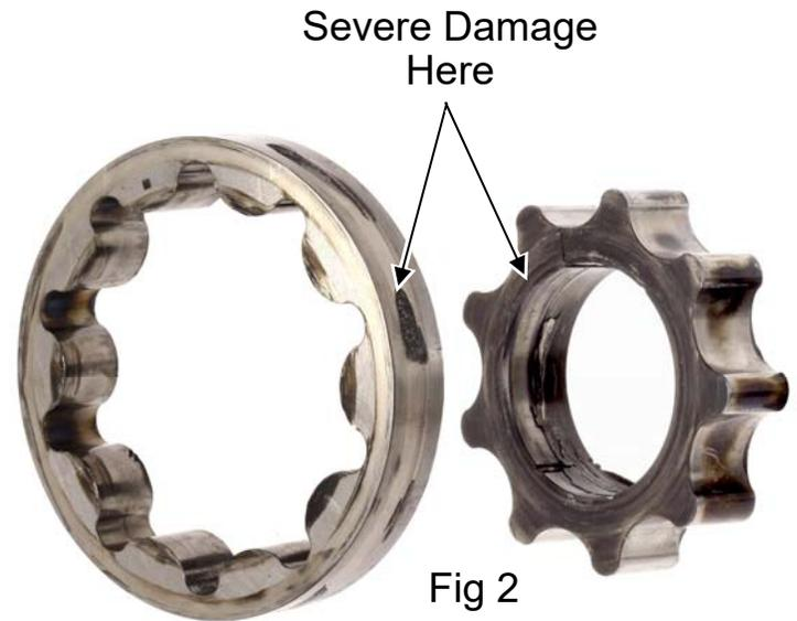
Lack of oil, restricted filter, dry start-up or aggressive TCM programming. Both gears are equally black & blued.
